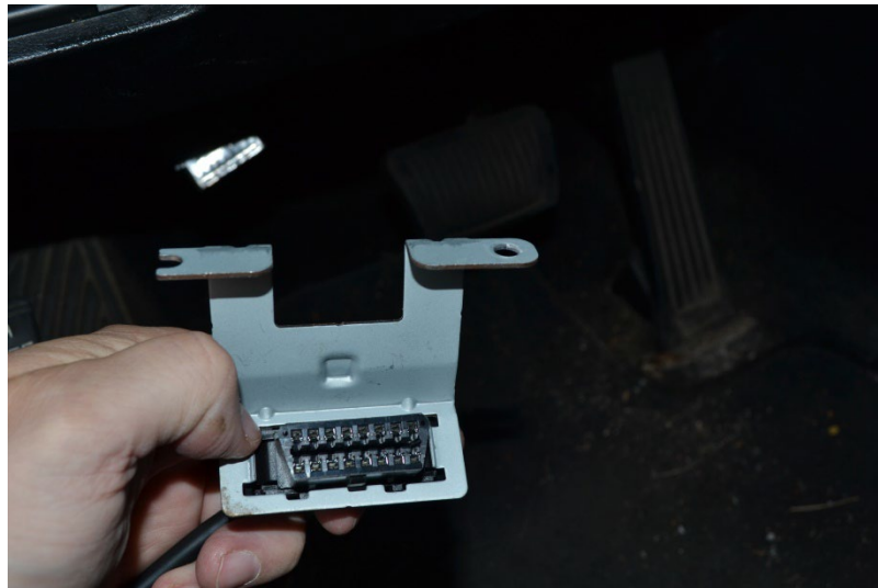
Figure 6 – The Y-Cable's OBD replica port inserted in bracket
