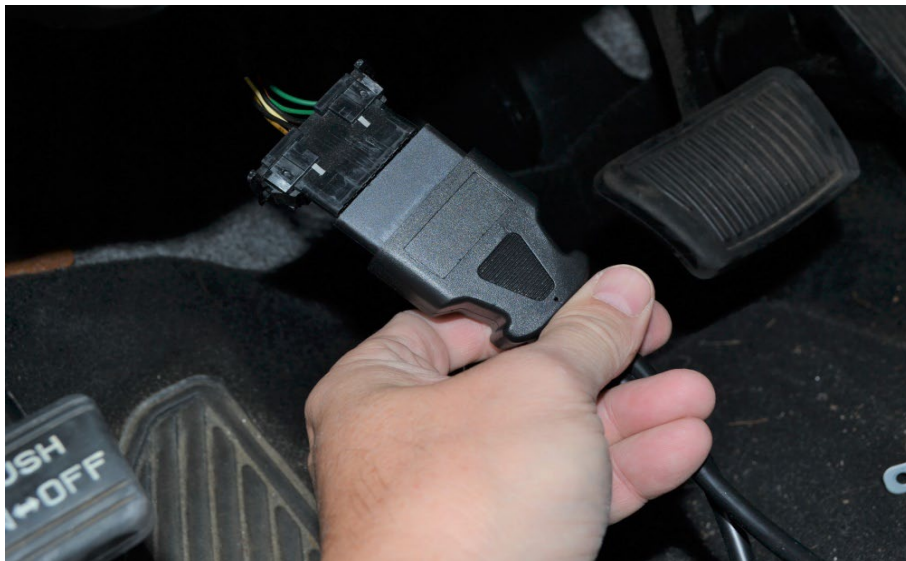
Figure 5 – Connecting Y-Cable to vehicle OBD port
