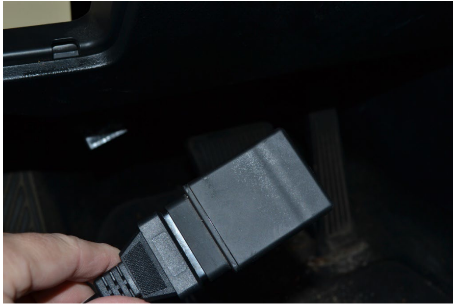
Figure 5 – Connecting GPS tracker to Y-Cable
