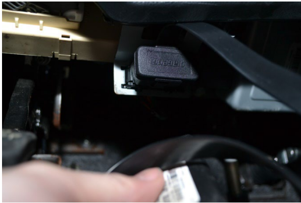
Plug male connector into OBDII port
