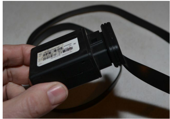
Plug female connector into tracker
