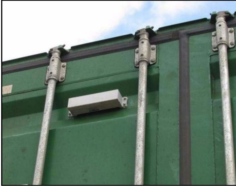
Top Left Container Door Mount (mounted in corrugation well between locking rods)
