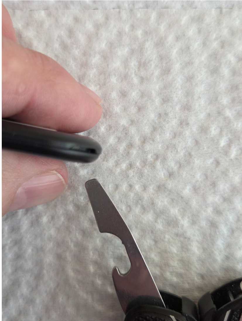
Pry the case open at the corner notch with a flat blade
