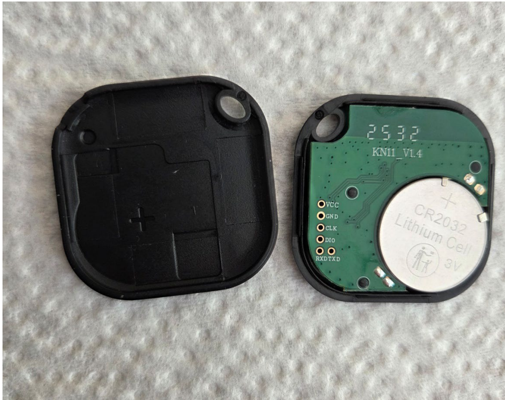
Opened tracker showing the PCB and CR2032 battery
